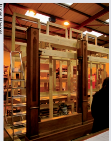
New frame for the organ incorporating some carved woodwork from the original.
